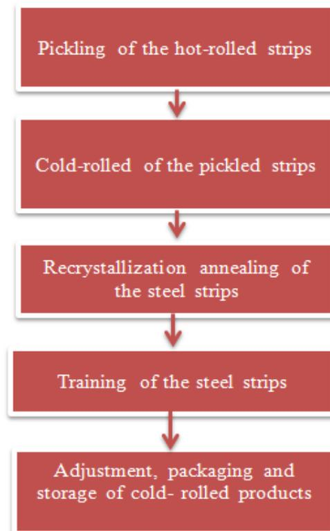
Fig. 1. Cold rolled steel manufacturing process
