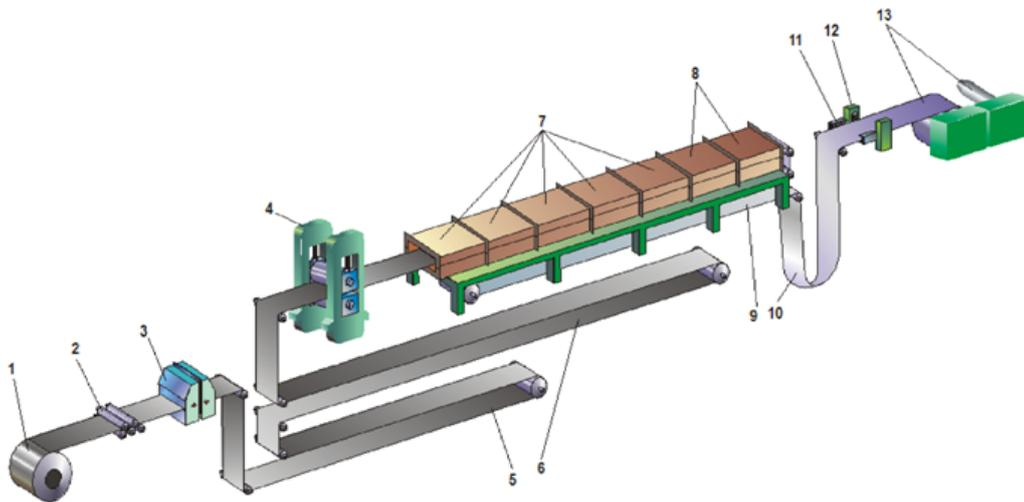
**Fig. 2.** Dip pickling line
